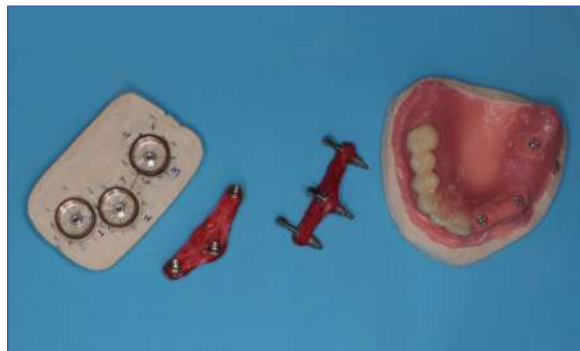
Figure 6. A customized Replica Production Device (RPD) utilized for the non-destructive negative replica technique implemented in this study. The RPD with three incorporated parallel implant analogs, identical to those utilized in the PRM, placed at the same relevant positions as the PRM and verified by two interchangeable verification jigs, one produced on the PRM and the other on the RPD.
