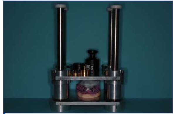
Figure 2. The pseudo-realistic model (PRM) with the seated tray placed under a constant axial load of 30N at an axial loading device (ALD) for 12min until the impression material was fully set.
