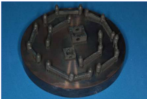
Figure 5. The parallel screw-retained Co-Cr bars manufactured on one plate by a computer aided manufacturing (CAM) - Selective Laser Melting (SLM) technique utilizing a 3D printer seen after the appropriate stress-relieving procedure.
