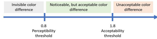
Figure 7. The shade tabs are divided into three groups based on the perceptibility and acceptability thresholds.
