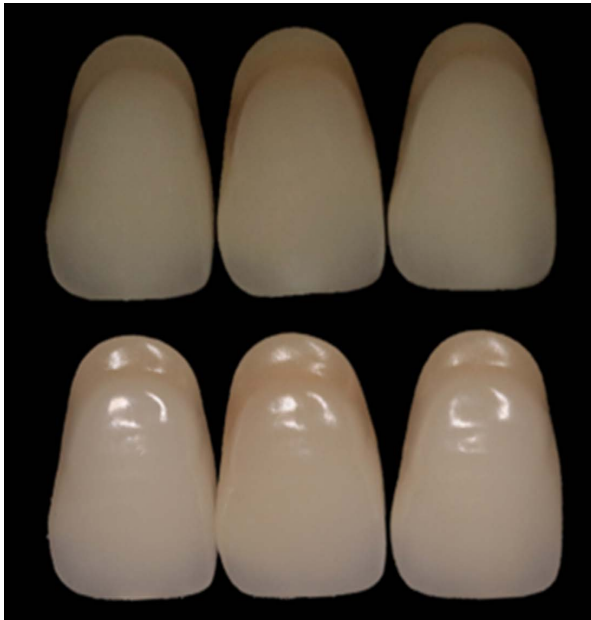
Figure 11. D2 shade tabs. Reference shade tab on the left side. Discolored shade tabs on the middle and on the right side. For the upper pictures a cross polarization filter was used to remove glare.
